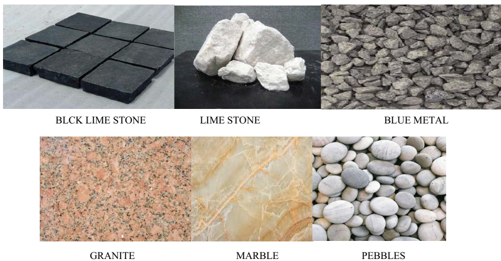
Fig. 9. Heat storage materials (black limestone, limestone, blue metal, granite, marble, pebbles).
