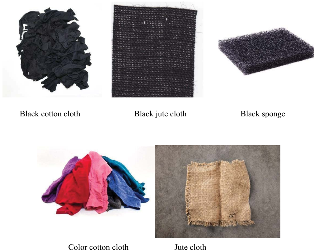
Fig. 14. Wick materials (black cotton cloth, black jute cloth, black sponge, color cotton cloth, jute cloth).
