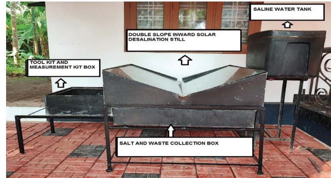
Fig. 3. V-type solar desalination still with experiment components.
