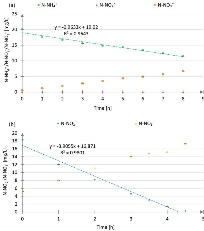
Fig. S3. N-NH<sub>4</sub><sup>+</sup>, N-NO<sub>2</sub><sup>-</sup>, N-NO<sub>3</sub><sup>-</sup> profiles during test (a) AUR-B and (b) NitUR-B. 1st repetition – 20°C.
