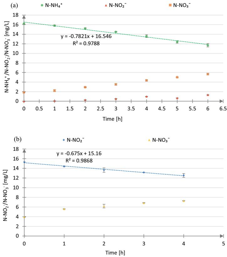
Fig. S11. N-NH<sub>4</sub><sup>+</sup>, N-NO<sub>2</sub><sup>-</sup>, N-NO<sub>3</sub><sup>-</sup> profiles during test (a) AUR-AS and (b) NitUR-AS. 2nd repetition – 12°C.
