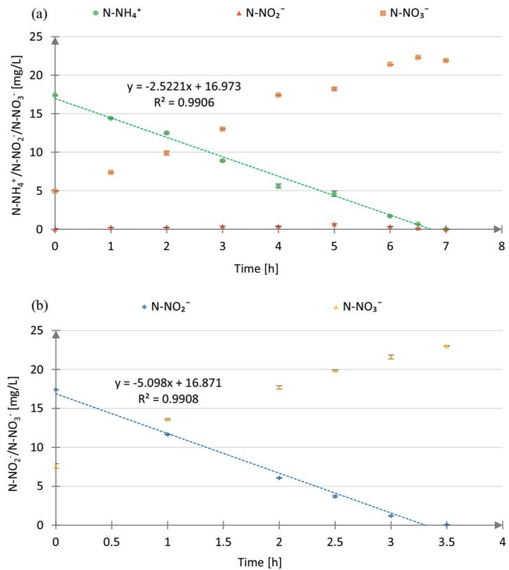
Fig. S4. N-NH<sub>4</sub><sup>+</sup>, N-NO<sub>2</sub><sup>-</sup>, N-NO<sub>3</sub><sup>-</sup> profiles during test (a) AUR-H and (b) NitUR-H. 2nd repetition – 20°C.
