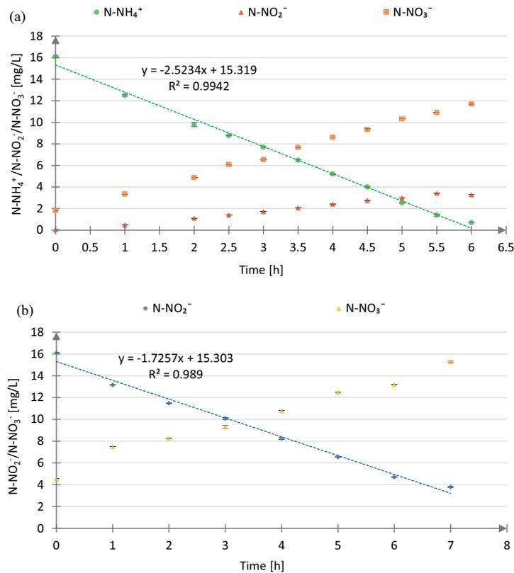
Fig. S2.  $N-NH_4^+$ ,  $N-NO_2^-$ ,  $N-NO_3^-$  profiles during test (a) AUR-AS and (b) NitUR-AS. 1st repetition – 20°C.
