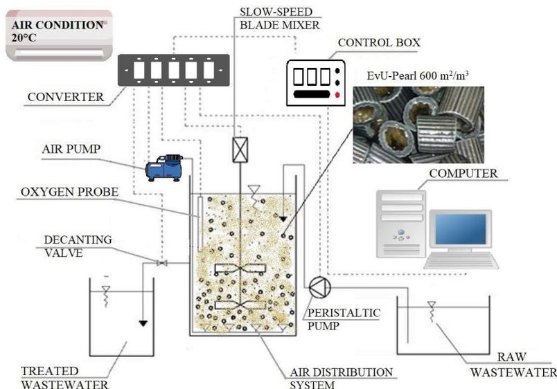
Fig. 1. Schematic of reactor with accessories.
