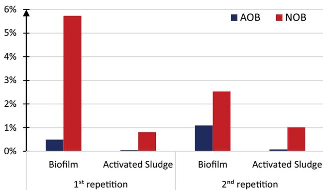
Fig. 2. Changes in the abundance of biofilm and activated sludge nitrifiers. Samples for new generation sequencing were taken from the main reactor working in 20°C. Graphs show the percentage contribution of AOB and NOB among all identified taxa.
