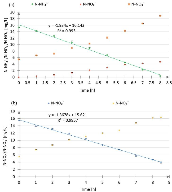
Fig. S5.  $N-NH_4^+$ ,  $N-NO_2^-$ ,  $N-NO_3^-$  profiles during test (a) AUR-AS and (b) NitUR-AS. 2nd repetition – 20°C.
