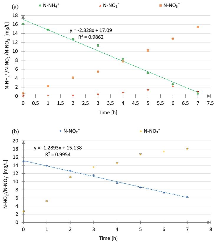
Fig. S8. N-NH<sub>4</sub><sup>+</sup>, N-NO<sub>2</sub><sup>-</sup>, N-NO<sub>3</sub><sup>-</sup> profiles during test (a) AUR-AS and (b) NitUR-AS. 1st repetition – 12°C.
