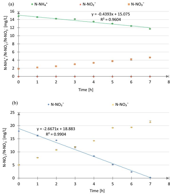
Fig. S9. N-NH<sub>4</sub><sup>+</sup>, N-NO<sub>2</sub><sup>-</sup>, N-NO<sub>3</sub><sup>-</sup> profiles during test (a) AUR-B and (b) NitUR-B. 1st repetition – 12°C.
