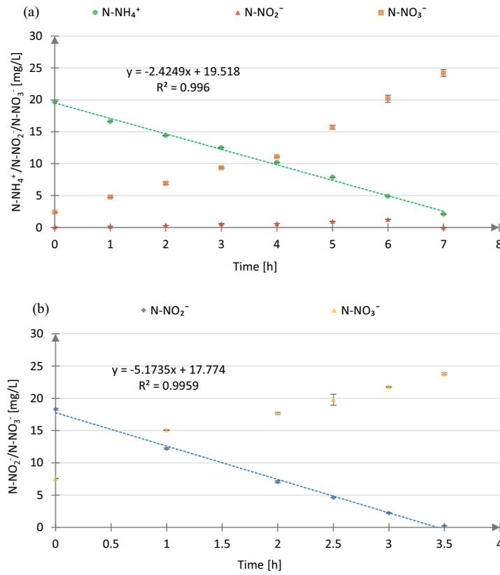
Fig. S7. N-NH<sub>4</sub><sup>+</sup>, N-NO<sub>2</sub><sup>-</sup>, N-NO<sub>3</sub><sup>-</sup> profiles during test (a) AUR-H and (b) NitUR-H. 1st repetition – 12°C.
