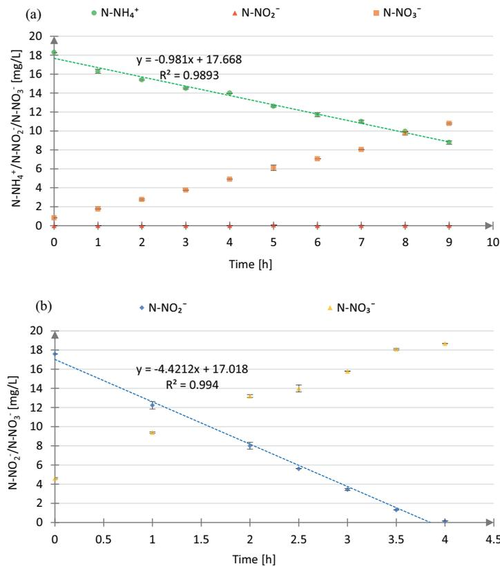
Fig. S6.  $N-NH_4^+$ ,  $N-NO_2^-$ ,  $N-NO_3^-$  profiles during test (a) AUR-B and (b) NitUR-B. 2nd repetition – 20°C.
