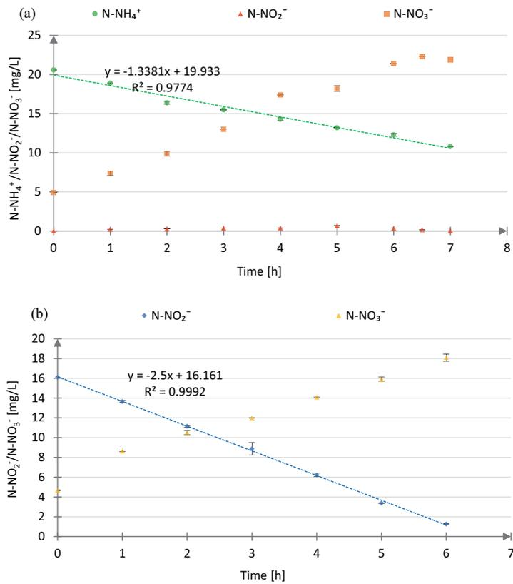
Fig. S10. N-NH<sub>4</sub><sup>+</sup>, N-NO<sub>2</sub><sup>-</sup>, N-NO<sub>3</sub><sup>-</sup> profiles during test (a) AUR-H and (b) NitUR-H. 2nd repetition – 12°C.
