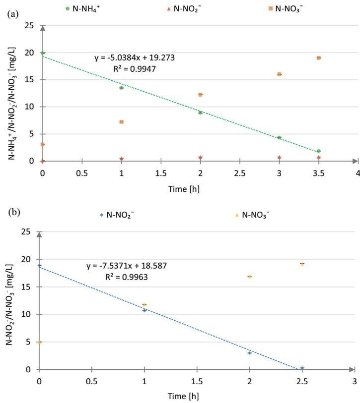
Fig. S1.  $N-NH_4^+$ ,  $N-NO_2^-$ ,  $N-NO_3^-$  profiles during test (a) AUR-H and (b) NitUR-H. 1st repetition – 20°C.
