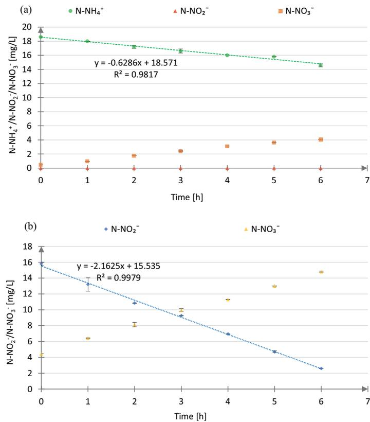
Fig. S12. N-NH<sub>4</sub><sup>+</sup>, N-NO<sub>2</sub><sup>-</sup>, N-NO<sub>3</sub><sup>-</sup> profiles during test (a) AUR-B and (b) NitUR-B. 2nd repetition – 12°C.
