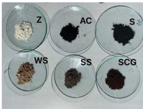
Fig. 1. Sorbents used within the landfill leachate pretreatment process Z – zeolite, AC – activated carbon, S – shungite, WS – walnut shells, SS – sewage sludge, SCG – spent coffee grounds.
