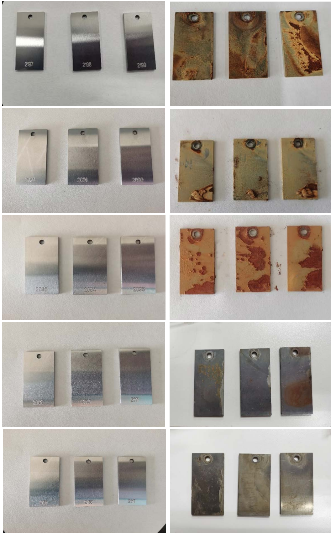
Fig. 6. Changes of some carbon steel sheets before and after reaction.
