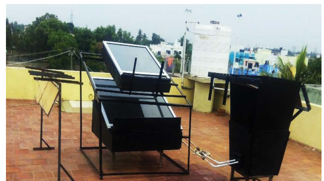
Fig. 1. Experimental set-up of double basin solar still integrated with solar pond.
