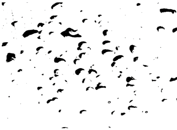
Fig. 27. Liquid flow rate: 12.5 L/min; gas flow rate: 2 L/min; projection depth: 27 cm; sparger diameter: 2mm; sparger opening: 4 (threshold view).
