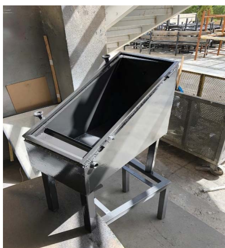
Fig. 2. Traditional solar purifier after manufacturing.
