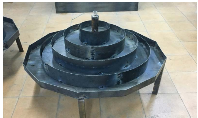
Fig. 4. Hemispherical still basin after manufacturing.
