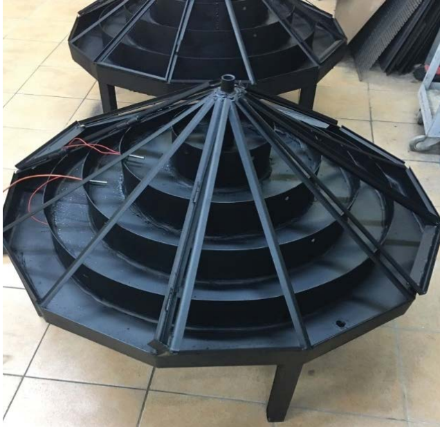
Fig. 7. Solar still with installed heaters.
