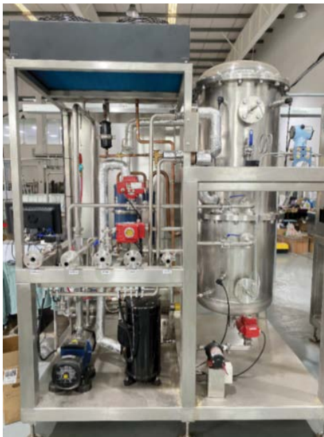
Fig. 4. Photograph of the tested single-effect heat pump desalination product.
