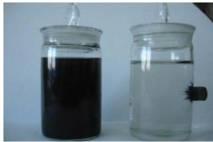
Fig. 8. Magnetism demonstration of \text{Fe}_3\text{O}_4/\text{maifan} stone.
