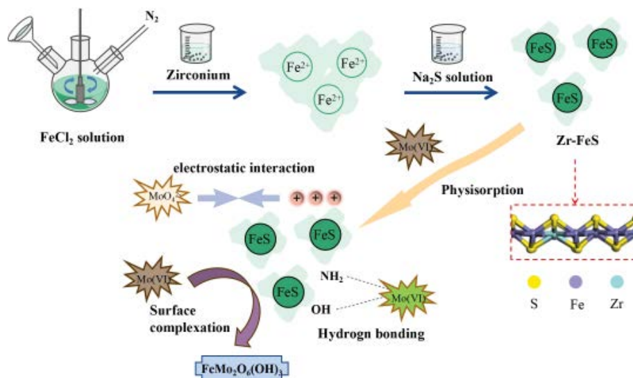
Fig. 10. Proposed mechanism for the adsorption of Mo(VI) onto Zr-FeS.
