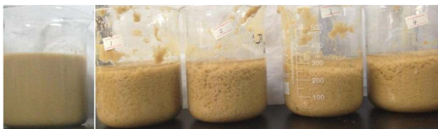
Fig. 6. Flocculation efficiency of mass ratio of konjac gum:orange peel (mass ratio of konjac gum:orange peel from left to right: 1:0, 1:1, 1:3, 1:5, 1:10).
