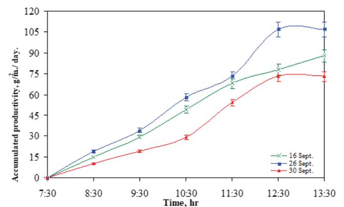
Fig. 12. Accumulated water productivity in test days.
