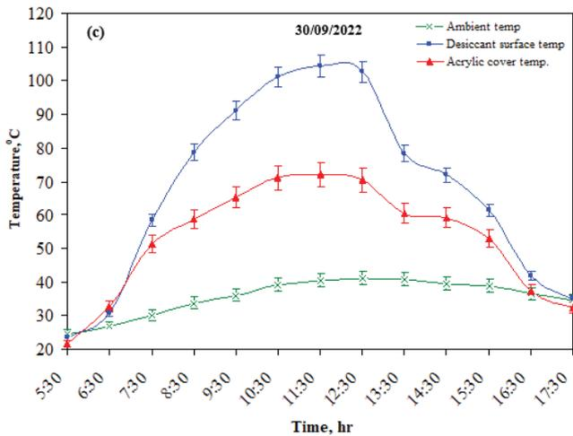
Fig. 8. Change of ambient, desiccant surface, and acrylic cover temperatures with time in (a) September 16, (b) September 26, and (c) September 30.
