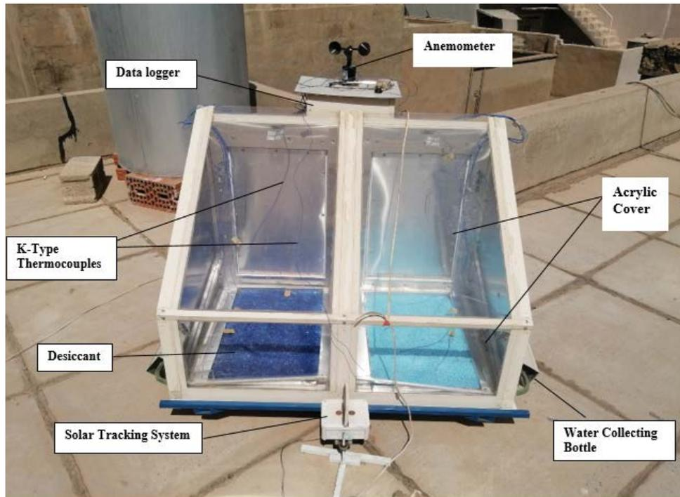
Fig. 1. Apparatus photograph.
