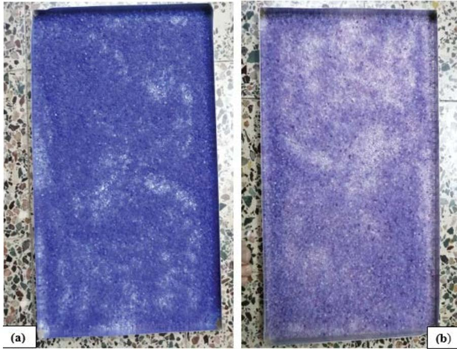
Fig. 3. Silica gel: (a) before moisture adsorption and (b) after moisture adsorption.
