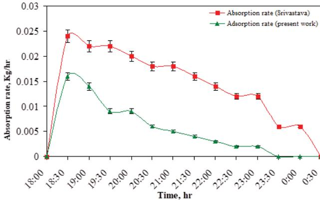
Fig. 5. Comparison of the adsorption rate of the present work with Srivastava and Yadav [6] work.
