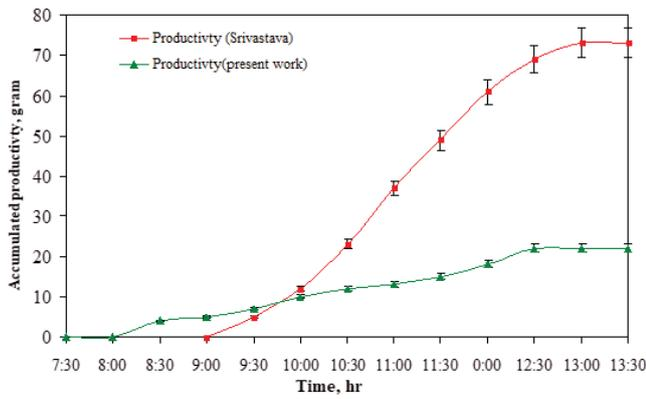
Fig. 6. Comparison of the accumulated water productivity of the current study with Srivastava and Yadav [6] work.
