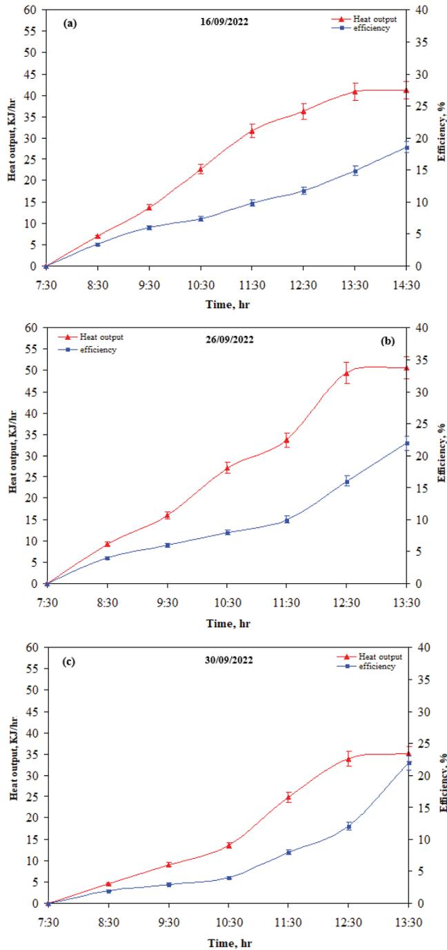
Fig. 13. Change of heat output and system efficiency with time in (a) September 16, (b) September 26, and (c) September 30.
