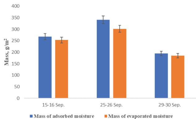
Fig. 10. Mass of adsorbed and evaporated moisture in various test days.
