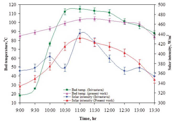
Fig. 4. Comparison of solar radiation and bed temperature of the present work with Srivastava and Yadav [6] work.
