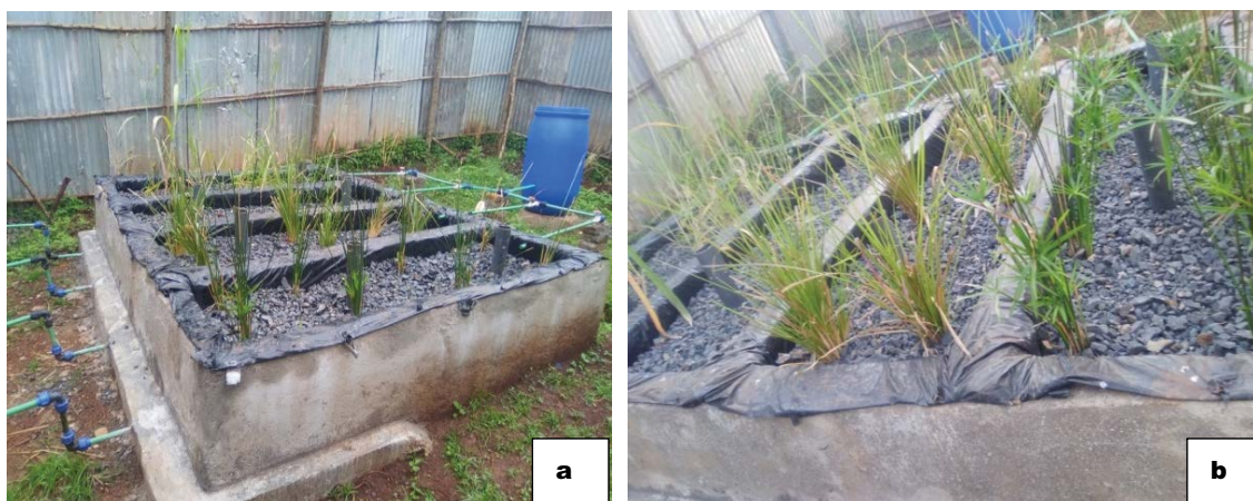
Fig. 7. Planted HSSFCW cells before (a) and after (b) feeding with pretreated WCPWW.
