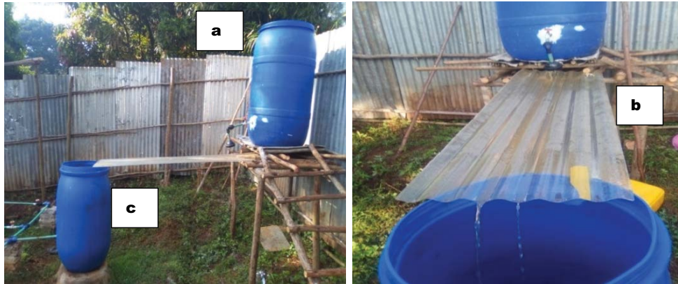
Fig. 2. Sedimentation (a), aeration (b), and equalization (c) processes.
