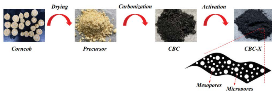
Fig. 1. Schematic illustration of the preparation process of CBC.
