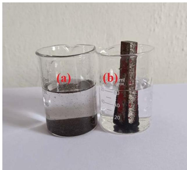
Fig. 12. MCSSC particles in Cd(II) solution, before (a) and after (b) magnetic separation.
