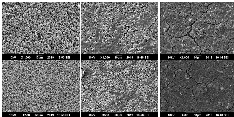
Fig. 10. (a) Virgin SDI filter, (b–c) used SDI filter (SDI > 5.0) at 500–1,000 magnification.
