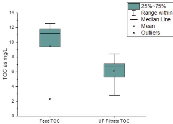
Fig. 9. Feed and UF filtrate total organic carbon.
