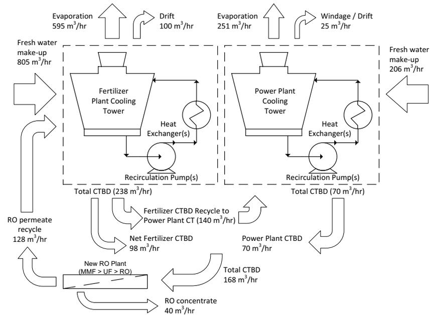
Fig. 2. Projected fertilizer plant mass balance and total CTBD generated for both systems.
