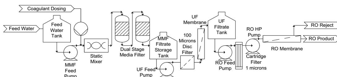
Fig. 3. Final treatment scheme for treating CTBD water.
