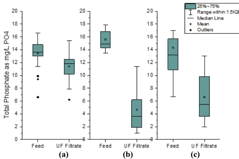
Fig. 11. Feed and UF filtrate total phosphate for (a) 0.02 μ UF, (b) 0.02 μ UF preceded by inline coagulation, and (c) 0.03 μ UF preceded by inline coagulation.
