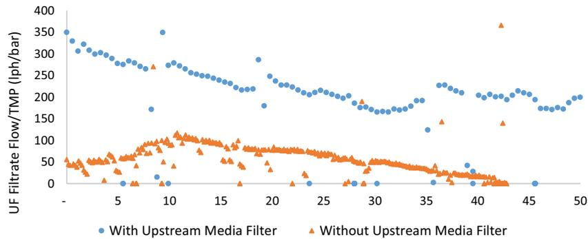
Fig. 12. Ultrafiltration filtrate flux (L/h·bar) decline with and without upstream media filter.
