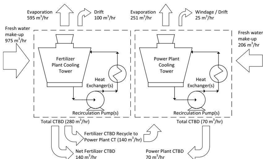
Fig. 1. Current fertilizer plant mass balance and total CTBD generated for both systems.
