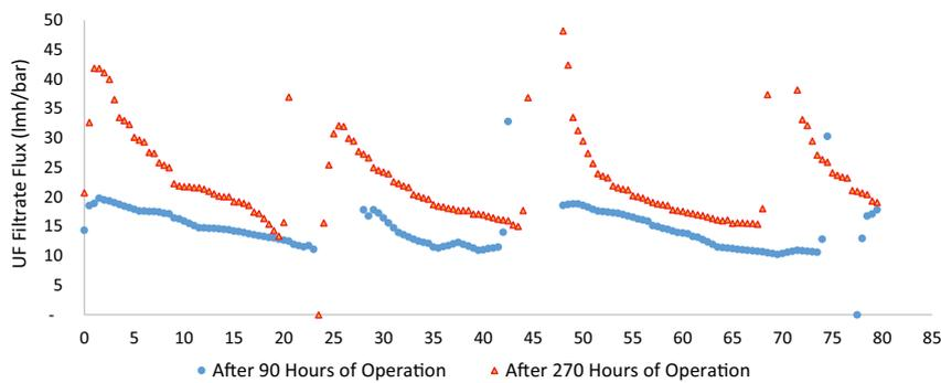
Fig. 13. Ultrafiltration filtrate flux (lmh·bar) profiles up to 270 h of operation.
