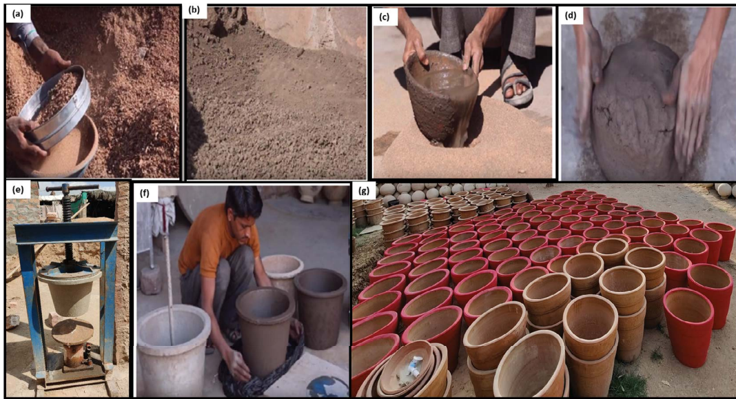
Fig. 1. (a) Sawdust (sieving), (b) clay, (c) wet mass preparation, (d) final consistency for green mould, (e) moulding machine, (f) frustum shaped filters and (g) final baked products.
