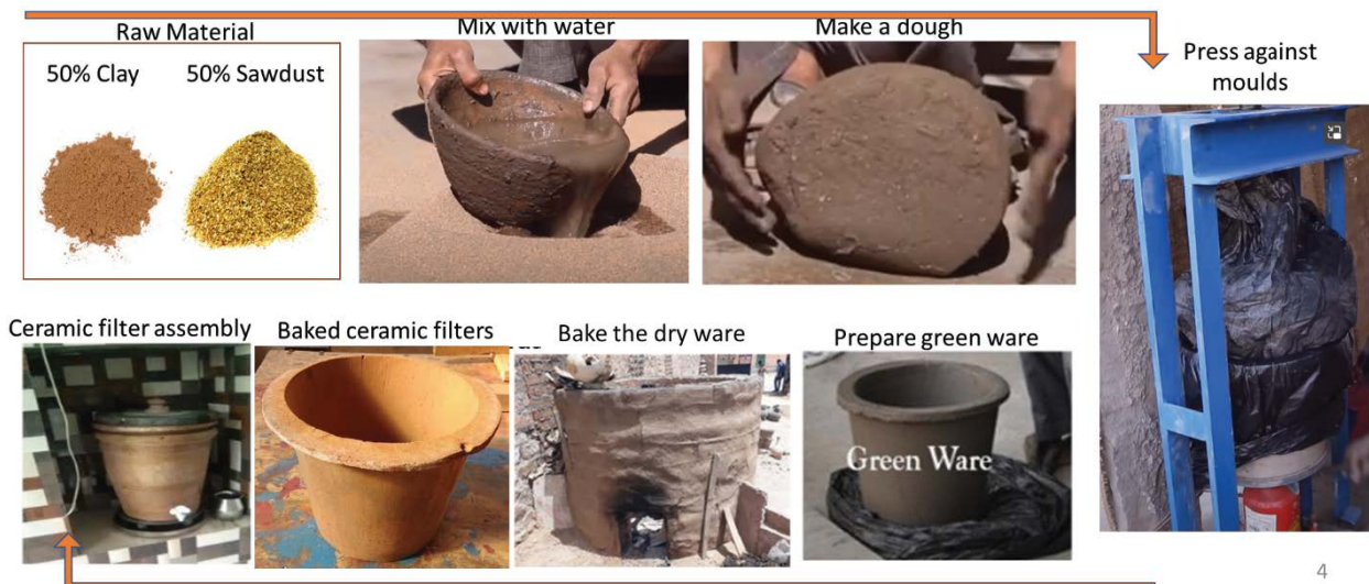
Fig. 1. Steps of ceramic filters manufacturing.
