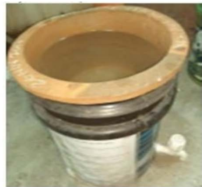
Fig. 2. G-filter receptacle in a clay container (Left). G-filter receptacle in a plastic container (Right) [14].
