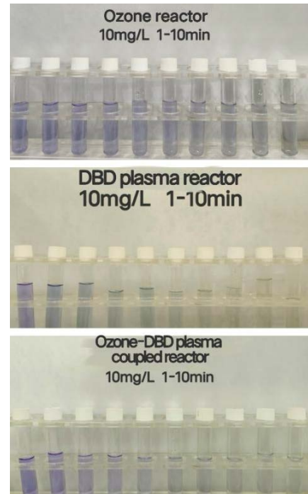
Fig. 17. Color change after degradation of crystalline violet solution treated with different reactors at pH = 7 with a discharge power of 150 W and an initial concentration of 10 mg/L.
