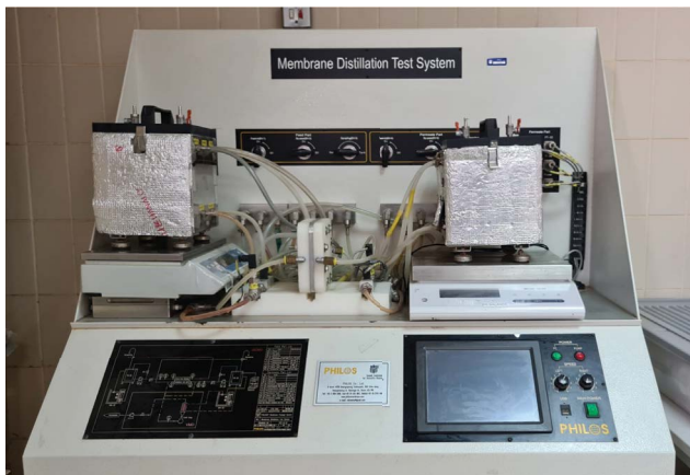
Fig. 2. Bench-scale direct contact membrane distillation (DCMD) test unit.
