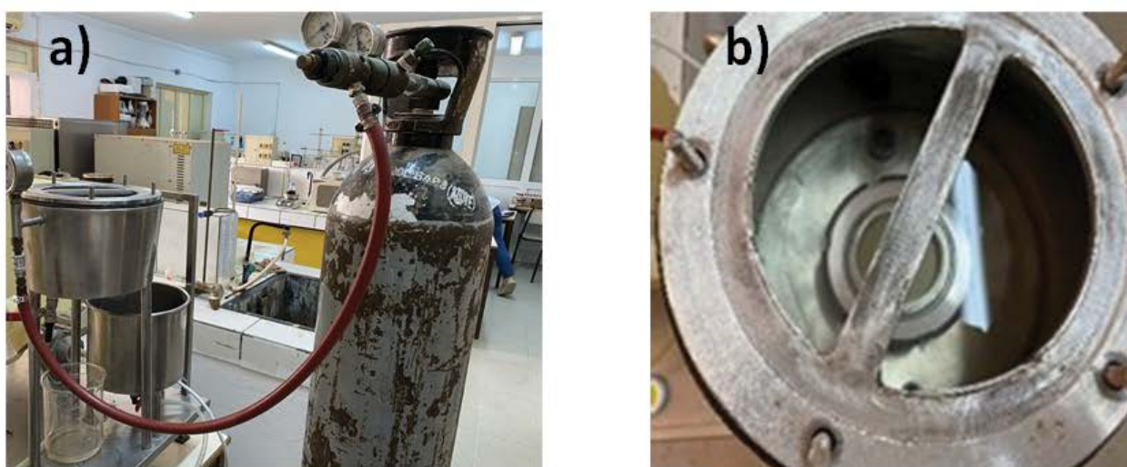
Fig. 3. (a) Laboratory filtration set-up and (b) flat disk membrane.
