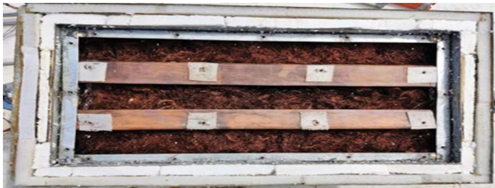
Fig. 3. Solar simulator box is filled with copper scraps at the bottom (Selvaraj et al. [30]).
