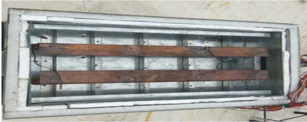
Fig. 2. Solar simulator is assembled with copper twin flat plates (Selvaraj et al. [30]).
