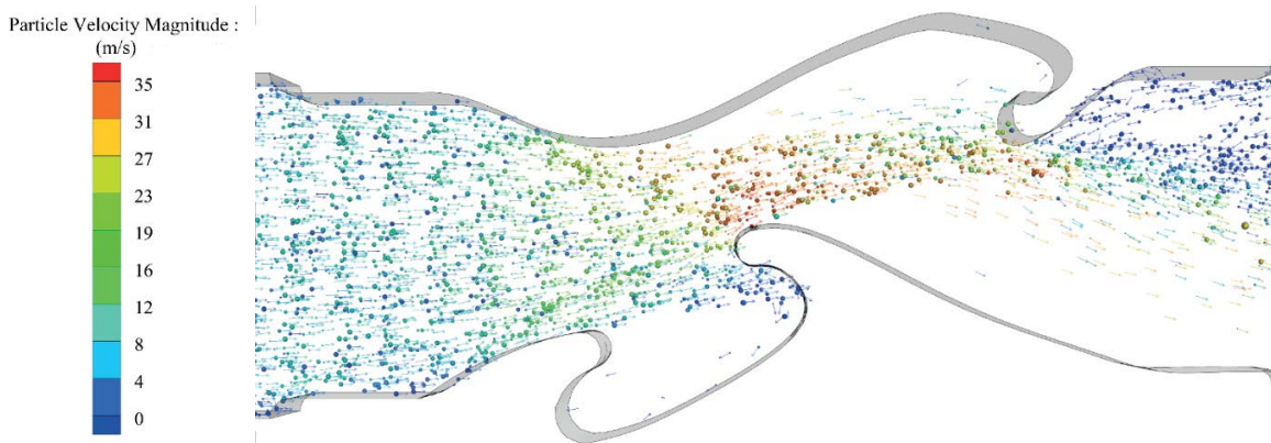
Fig. 19. Droplet tracking ( U_{in} = 9 m/s, I = 26 mm).
