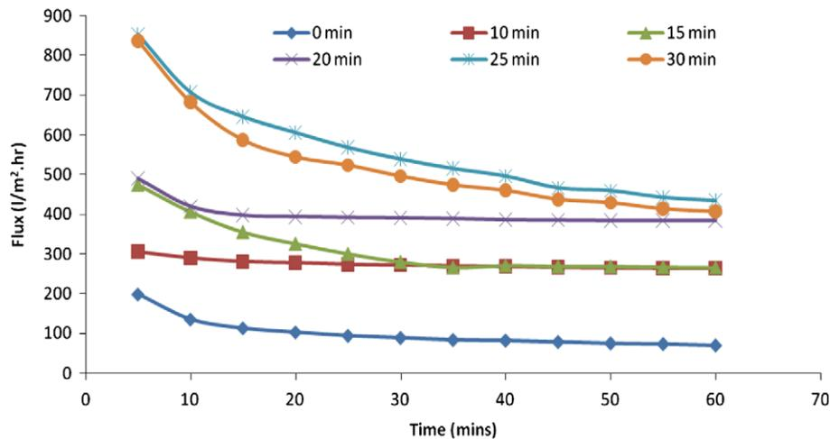
Fig. 4. Permeate flux with respect to time at various EC times (kaolin concentration = 400 mg/l, CV = 1.01/min).
