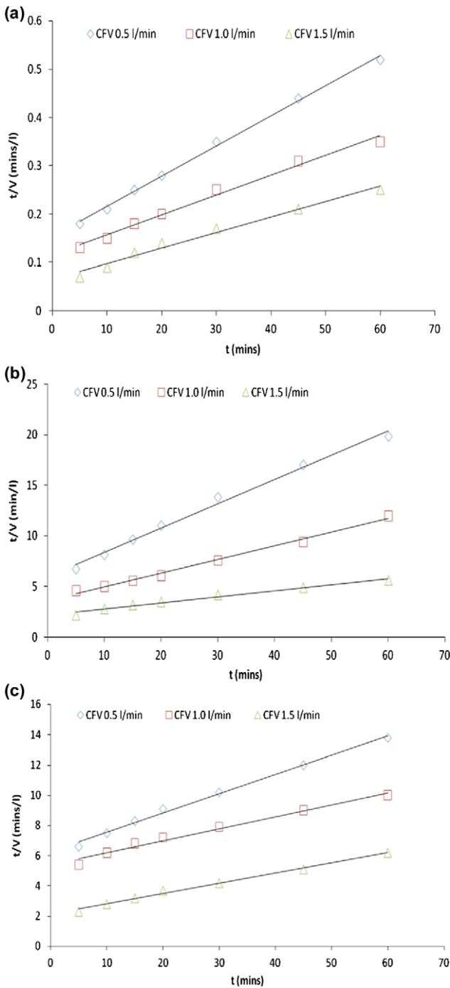
Fig. 3. Relationship between  $t/V$  and  $t$  for kaolin concentration of 800 mg/l at three different CVs.
