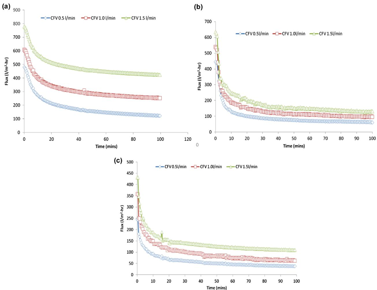
Fig. 2. Variation of crossflow MF flux with time at different crossflow velocities presented separately for different colloidal particle concentration (a) 100 mg/l kaolin, (b) 400 mg/l kaolin and (c) 800 mg/l kaolin.
