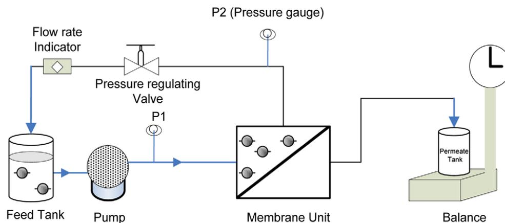
Fig. 1. Schematic diagram of the crossflow MF unit.
