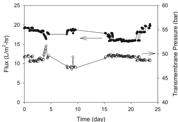
Fig. 3. Flux and transmembrane pressure for the SWRO pilot plant.
