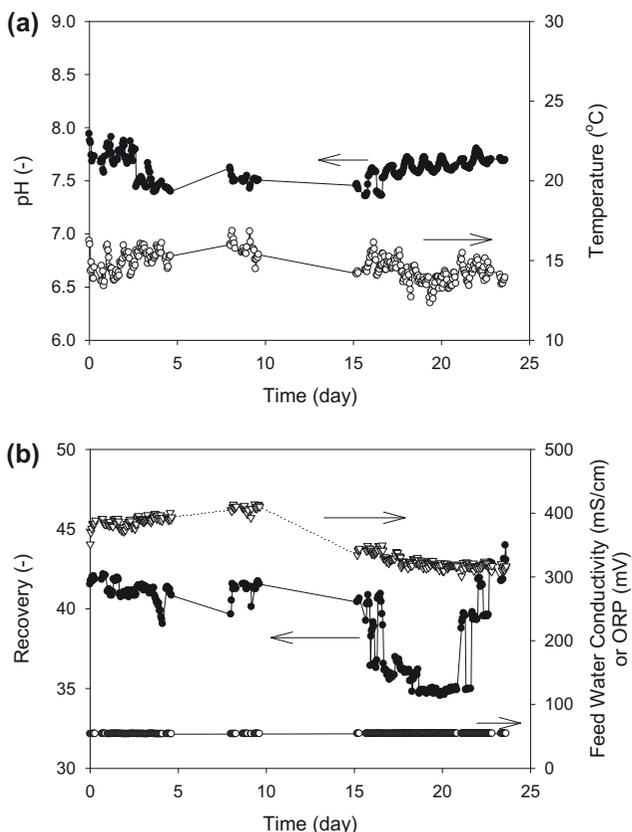
Fig. 2. Characteristics of feed water for the SWRO pilot plant. (a) pH and temperature and (b) conductivity, ORP, and recovery.
