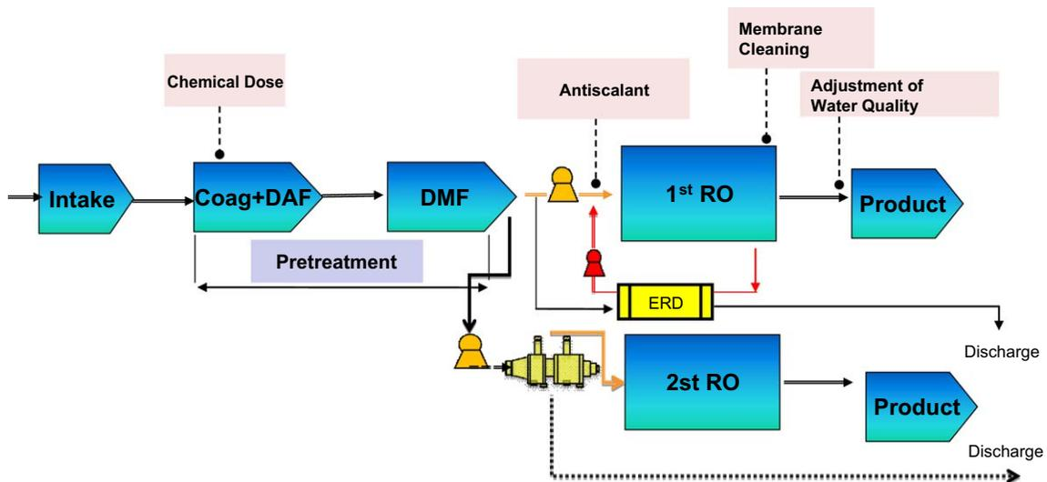
Fig. 1. Schematic diagram of the SWRO desalination pilot plant in Gijang, Korea.
