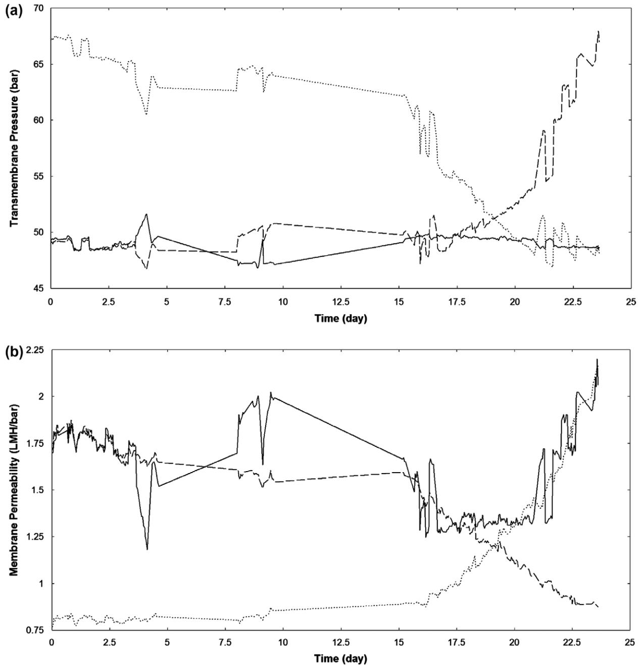
Fig. 5. Comparison of mathematical model fits with pilot plant data. (a) Transmembrane pressure and (b) Membrane permeability (—: pilot plant data; - - : mathematical model fitted to the early-stage data; ···: mathematical model fitted to the late-stage data).
