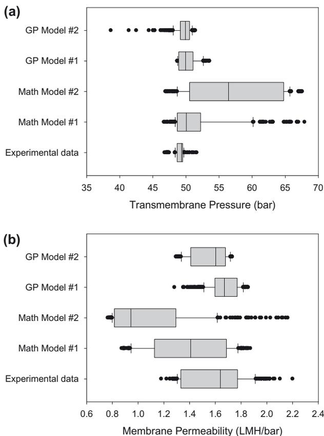
Fig. 8. Comparison of GP models with mathematical models. (a) Transmembrane pressure and (b) membrane permeability. Math models #1 and #2 were fitted to the early- and late-stage pilot plant data, respectively. GP models #1 and #2 were fitted to the early- and late-stage pilot plant data, respectively.
