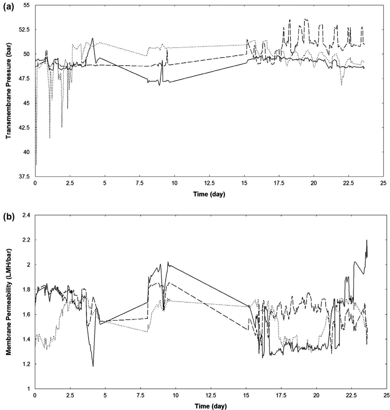
Fig. 7. Comparison of GP model fits with pilot plant data. (a) transmembrane pressure and (b) membrane permeability. (—: pilot plant data; - - : mathematical model fitted to the early-stage data; ··· : mathematical model fitted to the late-stage data).
