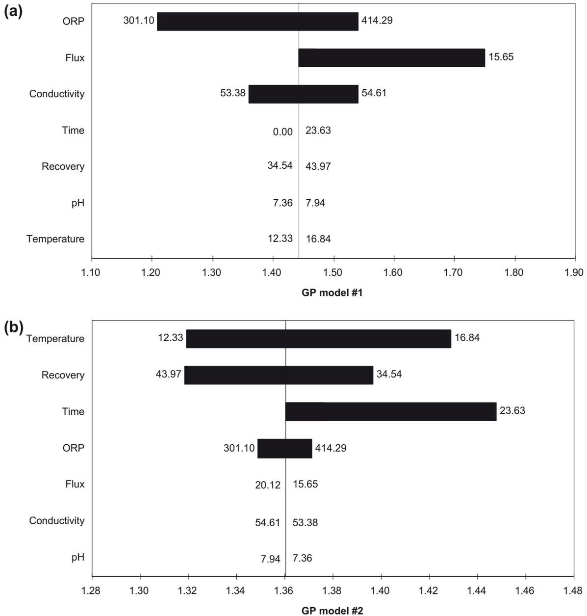
Fig. 9. Sensitivity analysis of the GP models. (a) GP model fitted to the early-stage data and (b) GP model fitted to the late-stage data.
