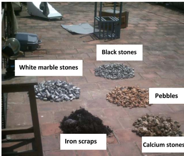
Fig. 2. Photograph of the sensible heat storage materials.
