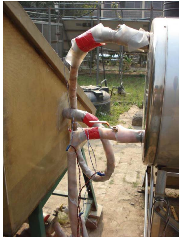
Fig. 2(a). A photograph of GI, plastic pipes, and thermocouples of EISS with insulation used to protect the heat loss during operation.
