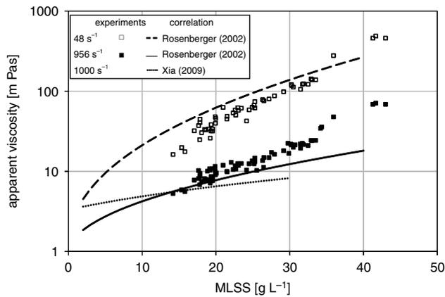
Fig. 3. Apparent viscosity at different shear rates for different MLSS concentrations.
