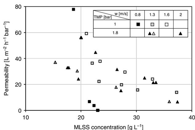
Fig. 5. Variation of permeability with MLSS concentration for different cross-flow velocities and transmembrane pressures.
