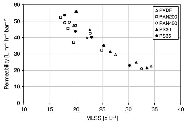
Fig. 4. Comparison of the permeability at different MLSS concentrations for various membrane materials under the same operational conditions (TMP = 1.8 ± 0.4 bar,  $w = 2 \pm 0.4 \text{ m s}^{-1}$ ).
