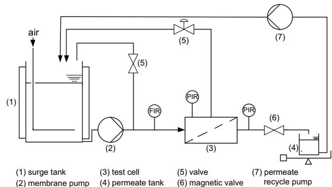
Fig. 1. Experimental set-up of the sludge thickening device.
