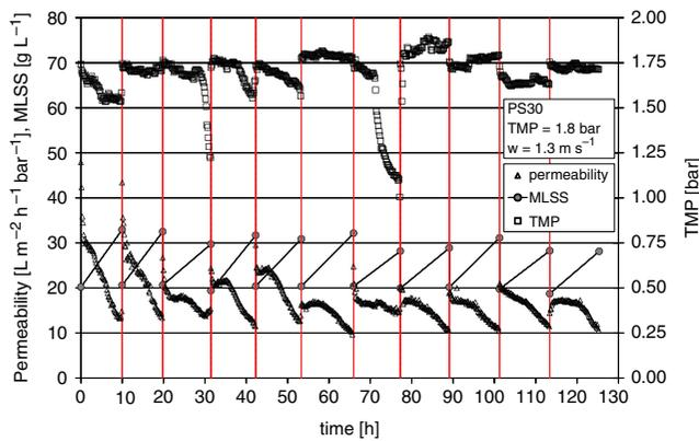
Fig. 7. Evolution of TMP, permeability and MLSS concentration over several successive thickening experiments.
