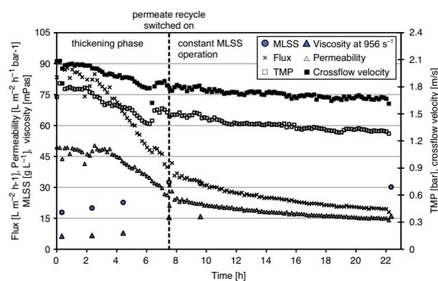
Fig. 2. Typical sludge thickening experiment and the characteristics of operational and process parameters.
