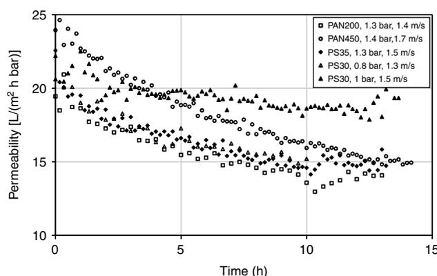
Fig. 6. Variation of permeability with time for continuous thickening at constant MLSS concentration.
