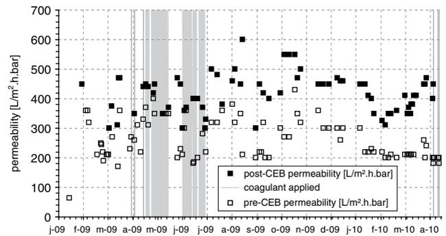
Fig. 3. UF permeability before and after CEB.
