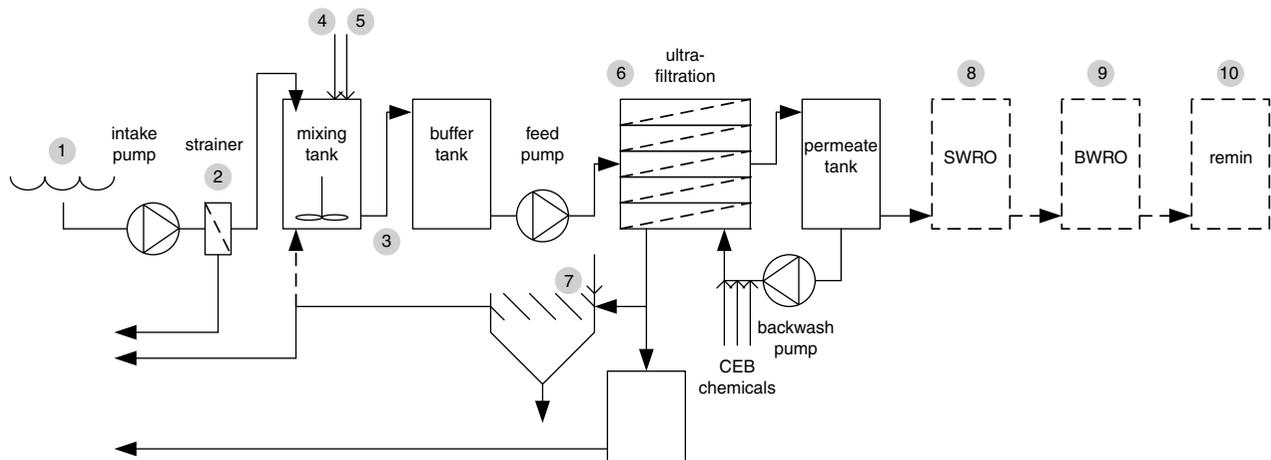
Fig. 1. Diagram Evides UF-SWRO demonstration plant.
