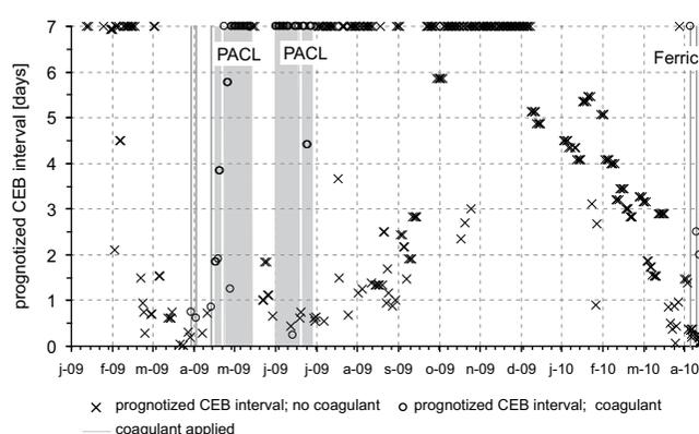
Fig. 5. CEB interval projected from initial permeability and permeability profile (cut-off at 7 d).
