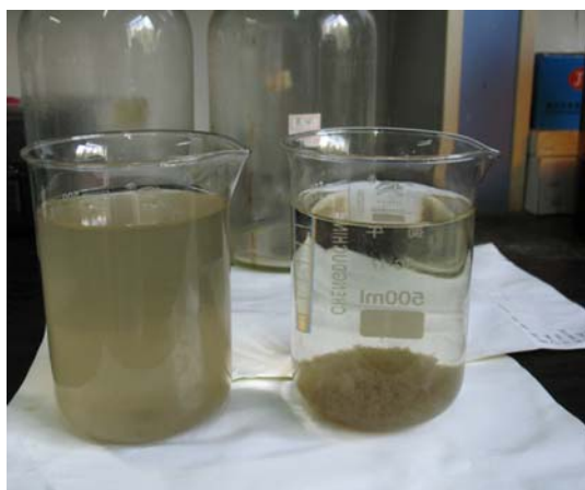
Fig. 2. Control of soybean protein wastewater with and without addition of PAC.
