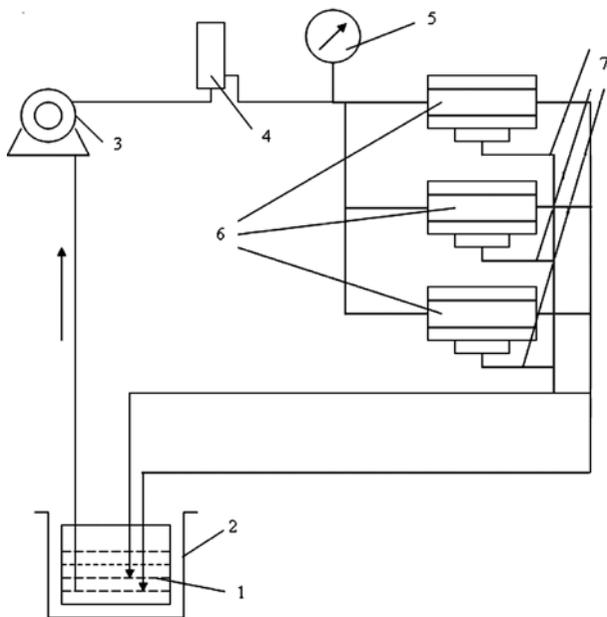
Fig. 1. Schematic view of laboratory facility with recycling solution: 1—container with recycling solution (artesian water or sodium chloride brine); 2—temperature regulator; 3—pump; 4—damping element; 5—pressure detector; 6—cells with membranes; and 7—permeate sampling.
