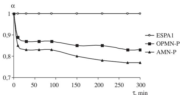
Fig. 5. The change of membranes' water flux in NF of artesian water with high carbonate hardness in the ACUMER presence ( $P=1.5$  MPa;  $v=1.5$   $\text{m s}^{-1}$ ; and  $T=21 \pm 1^\circ\text{C}$ ).
