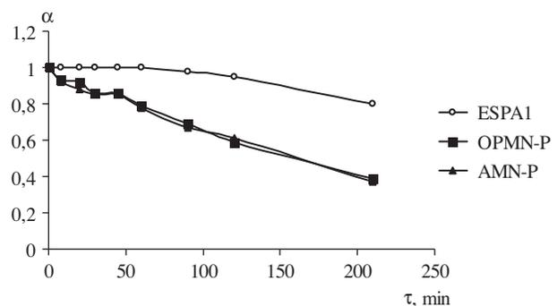
Fig. 3. The change of membranes' water flux in NF of artesian water with high carbonate hardness in absence of a scaling inhibitor ( $P = 1.5 \text{ MPa}$ ;  $v = 1.5 \text{ m s}^{-1}$ ; and  $T = 21 \pm 1^\circ \text{C}$ ).
