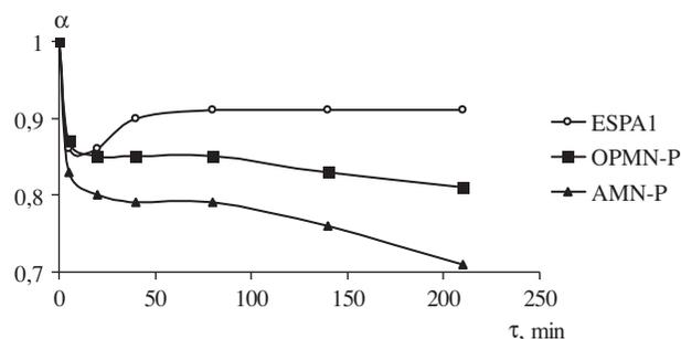
Fig. 4. The change of membranes' water flux in NF of artesian water with high carbonate hardness in the Na-CMC presence ( $P = 1.5$  MPa;  $v = 1.5$  m s<sup>-1</sup>; and  $T = 21 \pm 1$  °C).
