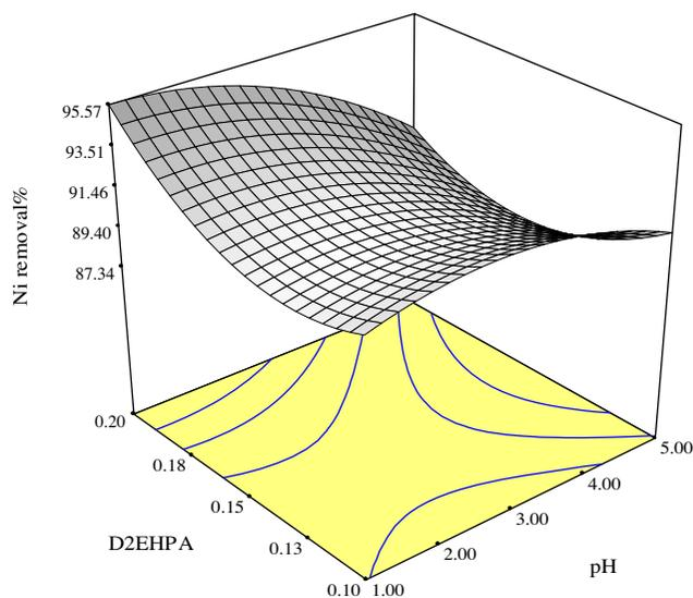
Fig. 1. Three-dimensional response surface for nickel removal as a function of pH and [D2EHPA].
