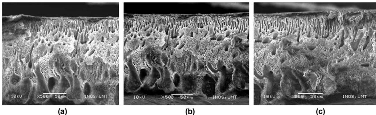
Fig. 3. SEM (1000 $\times$ ) cross sectional image of membranes: (a) MPH7-30, (b) MPH7-50, and (c) MPH7-70.
