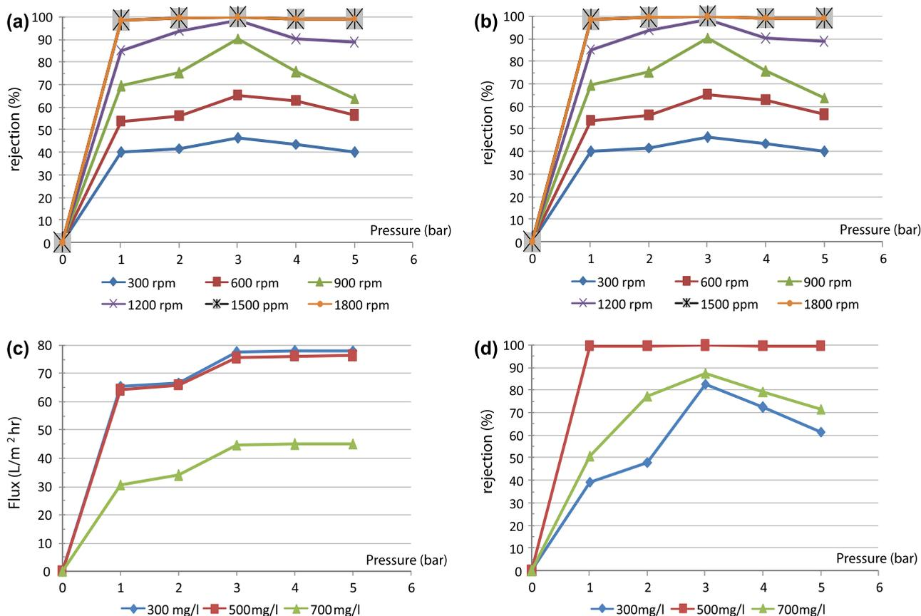
Fig. 5. Effect of stirring speed and feed concentration on MPH7-50 membrane flux and rejection profile at various pressure: (a) flux profile at various stirring speed, (b) rejection profile at various stirring speed, (c) flux profile at various feed concentration, and (d) rejection profile at various feed concentration.
