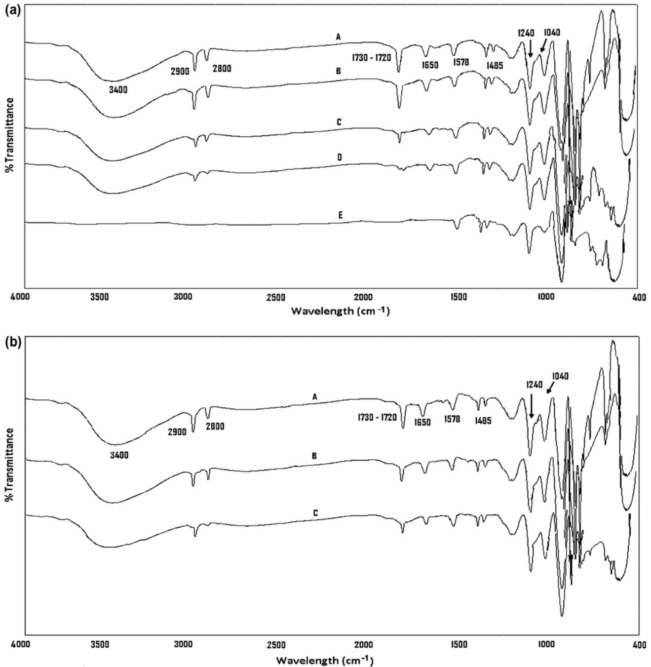
Fig. 1. FTIR spectra of (a) various pH, [A (MPH7) B (MPH5) C (MPH9) D (MPH11) & E (Native)] and (b) various myoglobin concentration [A (MPH7-50) B (MPH7-30) C (MPH7-70)].
