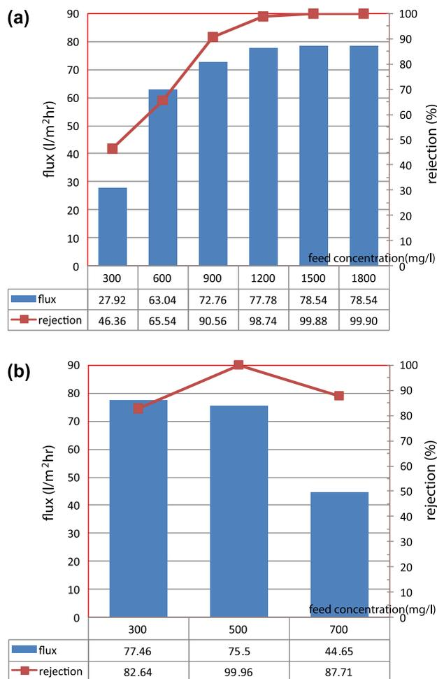
Fig. 6. Flux and rejection profile of feed concentration aMPH7-50 for operating pressure of 3 bar at various (a) stirring speed and (b) myoglobin concentration.
