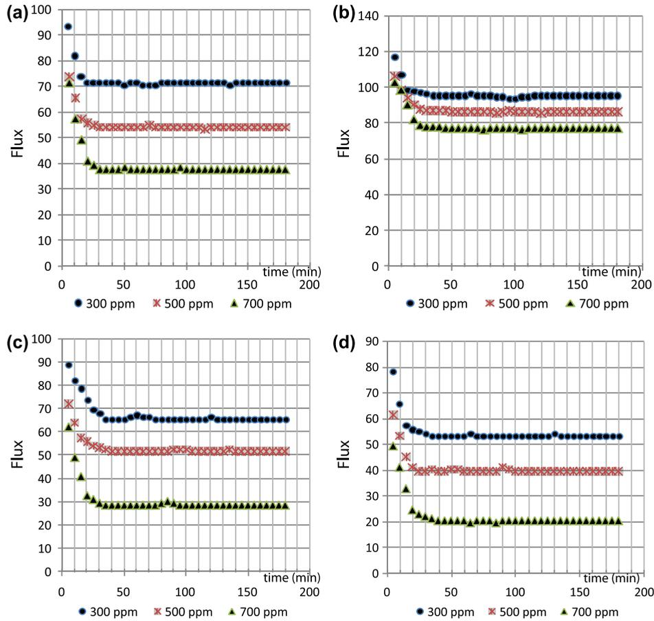
Fig. 4. Flux profile as a function of time for myoglobin-coated membranes at various pH and feed concentration: (a) MPH-5, (b) MPH-7, (c) MPH-9, and (d) MPH-11.
