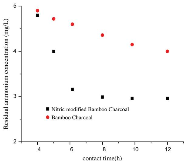
Fig. 3. Effect of contact time on the removal of ammonium (pH: 7; initial ammonium concentration: 5 mg/L; temperature: 5°C).
