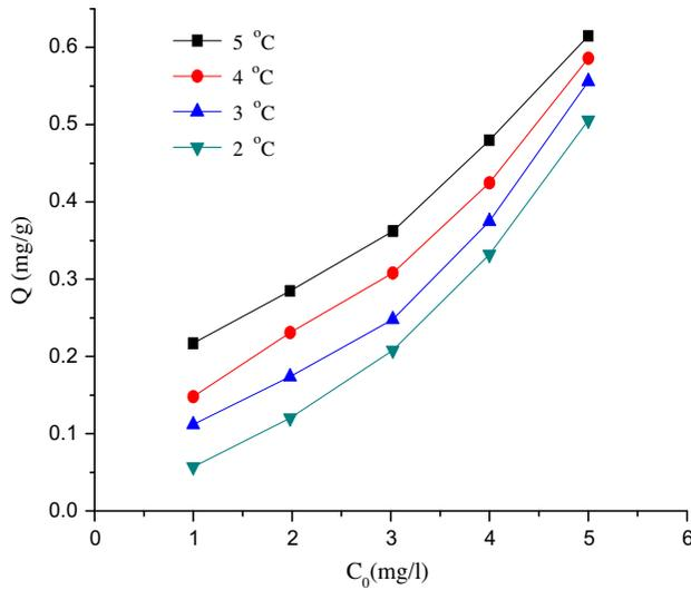
Fig. 6. Effect of initial ammonium concentration on the removal of ammonium (contact time: 360 min; pH: 7; adsorbent dosage: 1 g/L; temperature: 1–5 °C).
