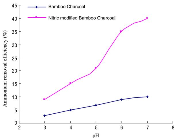
Fig. 4. Effect of pH on the removal of ammonium (adsorbent dosage: 1 g/L; contact time: 360 min; initial ammonium concentration: 5 mg/L; temperature: 5°C).
