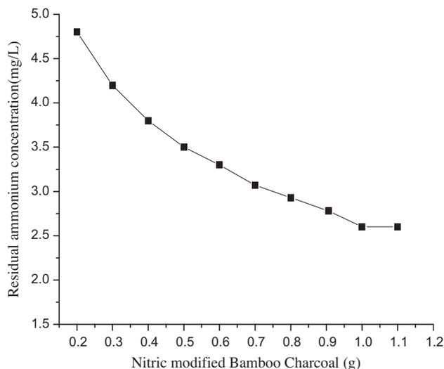
Fig. 5. Effect of adsorbent dosage on the removal of ammonium (contact time: 360 min; pH: 7; initial ammonium concentration: 5 mg/L; temperature: 5°C).
