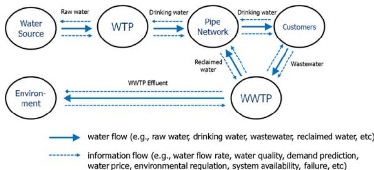
Fig. 1. The water and information flow diagram in a smart water grid.
