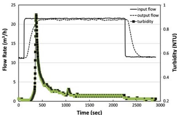
Fig. 3. The turbidity of the supernatant water (output) in the sedimentation process in the pilot-scale system according to the flow rate fluctuation.
