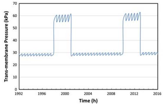
(b) Case 2: variable flux operation at 1.6 m/d for peak time and 0.8 m/d for ordinary time
