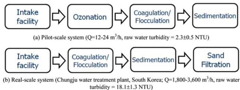
Fig. 2. The flow diagrams of two conventional water treatment systems for this study.
