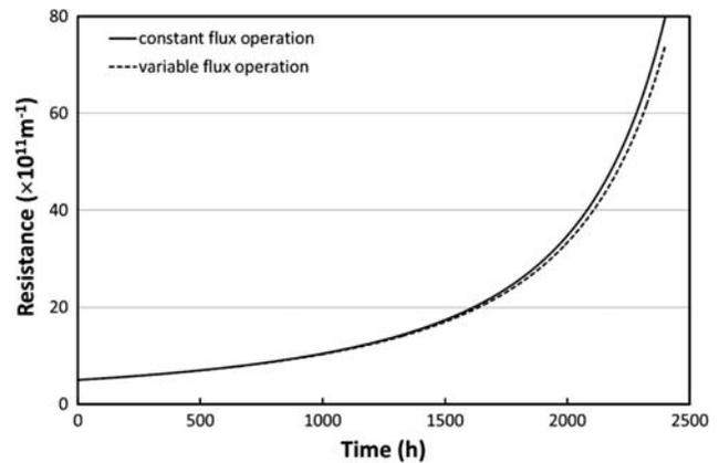
Fig. 7. Changes of total membrane resistance for 100 days of the MF simulation.
