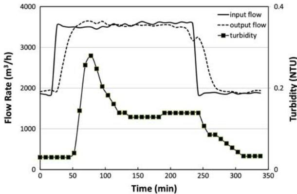
Fig. 4. Turbidity of filtrate (output) from the sand filtration in the real-scale system according to the flow rate fluctuation.
