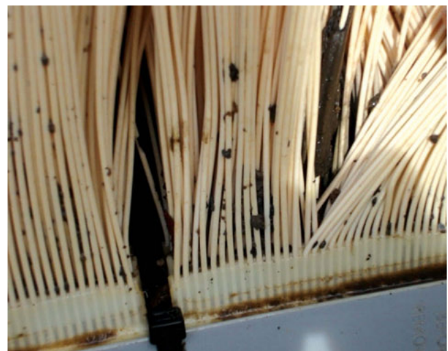
Fig. 7. Bottom part of the membrane module, taken at the end of the operational period.
