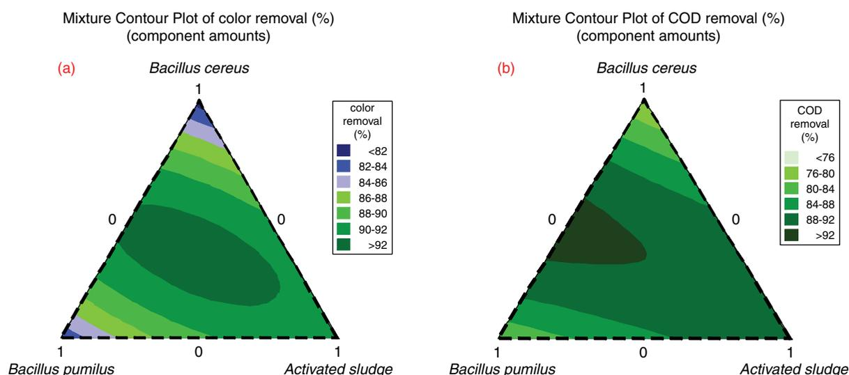
Fig. 1. Mixture contour plots between the variables (*Bacillus cereus*, *Bacillus pumilus*, and activated sludge) for colour (a) and COD (b) removal (%).
