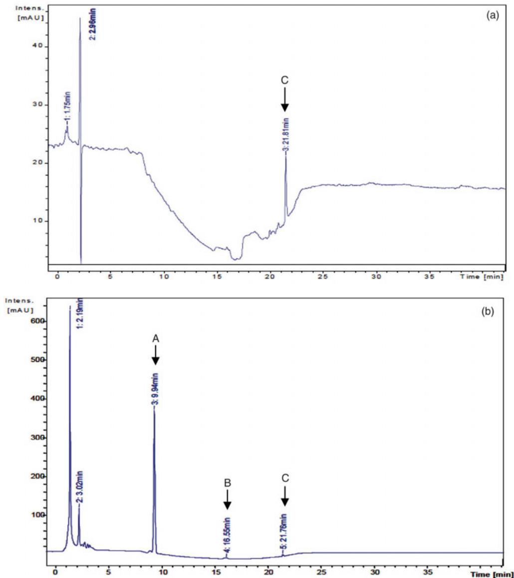
Fig. 2. HPLC spectra of the textile wastewater containing indigo dye before (a) and after degradation (b) by 33% *Bacillus cereus*, 33% *Bacillus pumilus* and 33% activated sludge (48 h of incubation).
