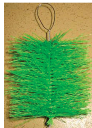
Fig. 2. A three-dimensional elastic carrier made from PET.
