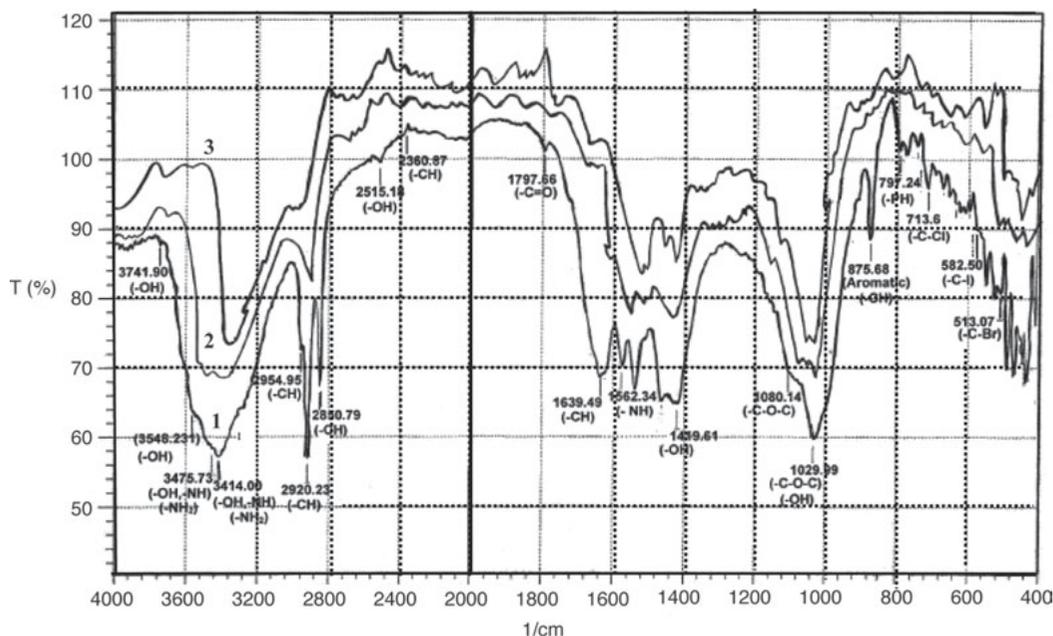
Fig.1. FT-IR spectra of dead microorganisms (1) before phenol and lead biosorption (2) after phenol biosorption (3) after lead biosorption.
