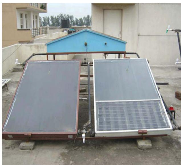
Fig. 1b. Photograph of HPVT double slope active solar still.
