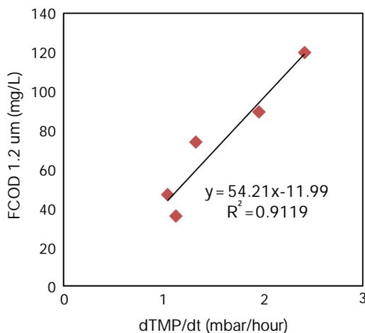
Fig. 4. Correlation between membrane fouling rate and FCOD in BF-MBR.
