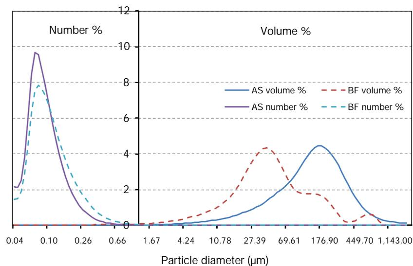
Fig. 7. Comparing of particle size distribution (PSD) between AS-MBR and BF-MBR membrane feed solutions.
