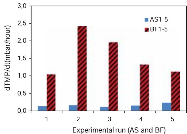
Fig. 2. Membrane fouling rate of the BF-MBR and AS-MBR.
