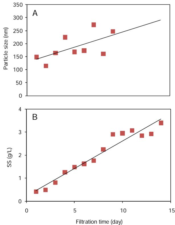
Fig. 10. Variation of submicron particle size when SS increasing in BF-MBR
