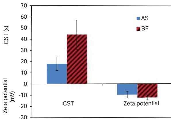
Fig. 5. Comparison of CST and zeta potential between the AS-MBR and BF-MBR.
