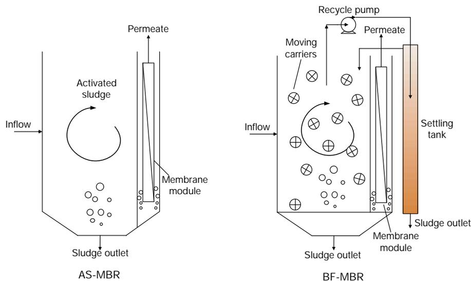
Fig. 1. System configuration of the AS-MBR and BF-MBR pilot plants.
