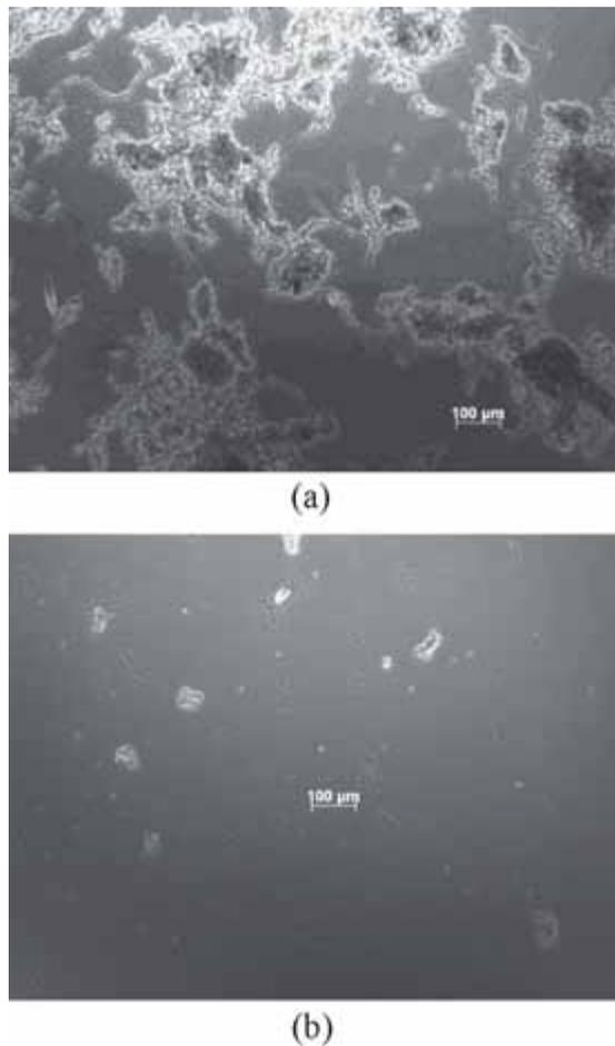
Fig. 6. Microscope pictures of (a) activated sludge flocs, and (b) biofilm flocs.
