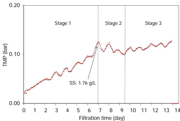
Fig. 8. TMP profile of increasing SS in the BF-MBR, test BF6.
