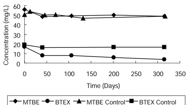
Fig. 4. Degradation of MTBE and BTEX by aquifer sediments under nitrate reduction condition.
