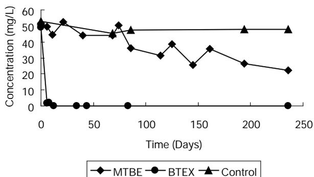
Fig. 2. Degradation of MTBE and BTEX by microorganisms extracted from aquifer sediments under aerobic condition.
