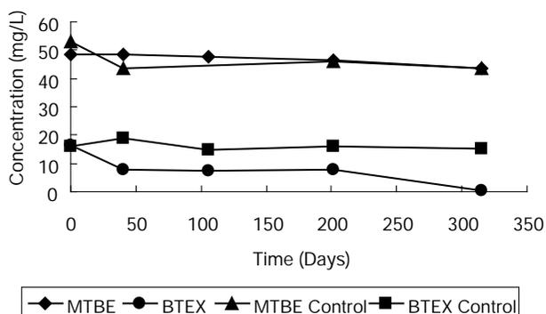
Fig. 5. Degradation of MTBE and BTEX by aquifer sediments under methanogenesis condition.
