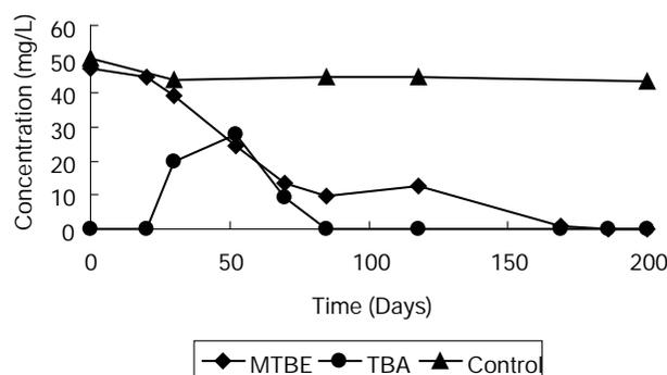
Fig. 1. Degradation of MTBE by aquifer sediments under aerobic condition.
