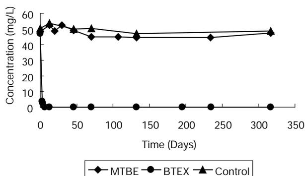
Fig. 3. Degradation of MTBE and BTEX by activated sludge under aerobic condition.
