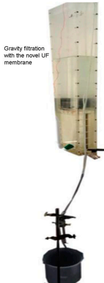
Fig. 7. Gravity filtration design made in Australia.
