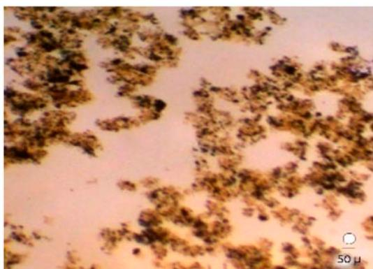
Fig. 5. Micrograph of flocs for synthetic oily water.
