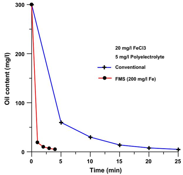
Fig. 3. Oil content variation during settling for synthetic oily water.
