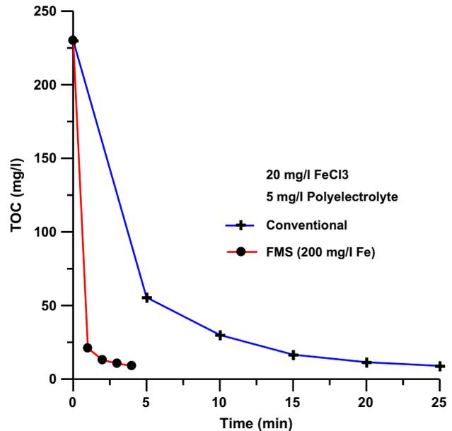
Fig. 4. TOC variation during settling for synthetic oily water.
