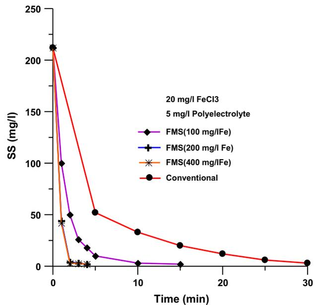
Fig. 1. SS variation during settling for synthetic oily water using different ferromagnetic particles doses.
