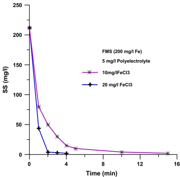
Fig. 2. SS variation during settling for synthetic oily water using two different coagulant doses.
