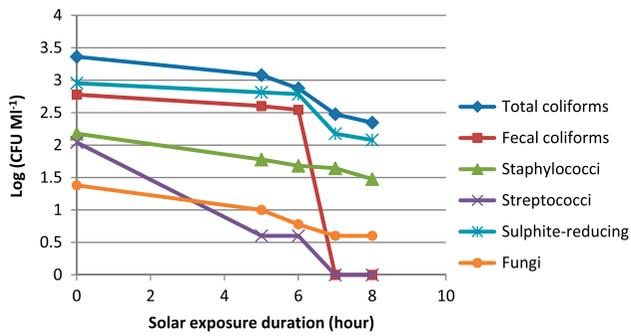
Fig. 4. Temporal evolution of secondary-treated wastewater disinfection using solar photolysis.
