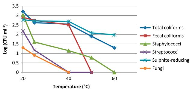
Fig. 5. Evolution of secondary-treated wastewater disinfection using solar photolysis under the heating effect.
