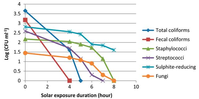
Fig. 8. Performance evaluation of the 50 L plan photoreactor used for a secondary-treated wastewater disinfection by solar photolysis.
