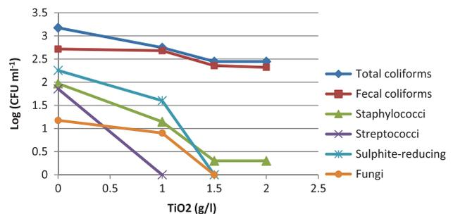
Fig. 6. Evolution of secondary-treated wastewater disinfection using photocatalysis under  $\text{TiO}_2$  concentrations.
