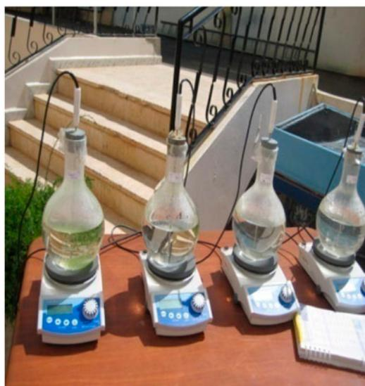
Fig. 1. Photolysis test bench.
