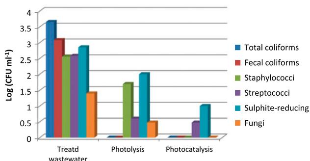
Fig. 7. Comparative study of the photolysis and photocatalysis processes used for secondary-treated wastewater disinfection.
