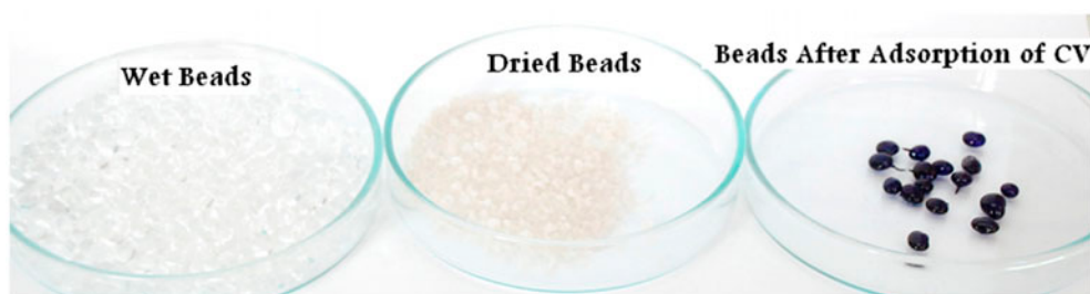
Fig. 1. Photographs of wet and dried carrageenan beads and carrageenan beads after adsorption of CV.
