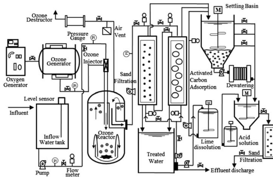
Fig. 1. Schematic of the pilot-scale plant for the removal of iron and manganese ions from abandoned NAMD via ozone oxidation and micro-sand filtration.
