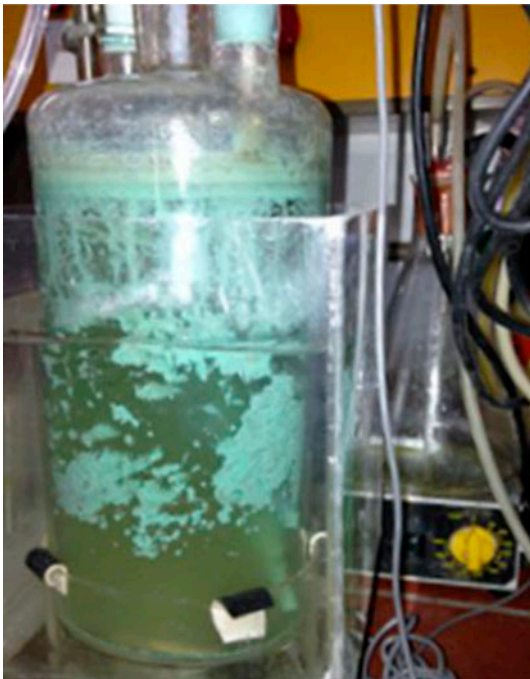
Fig. 4. Formation of biofilm on the walls of the bioreactor.
