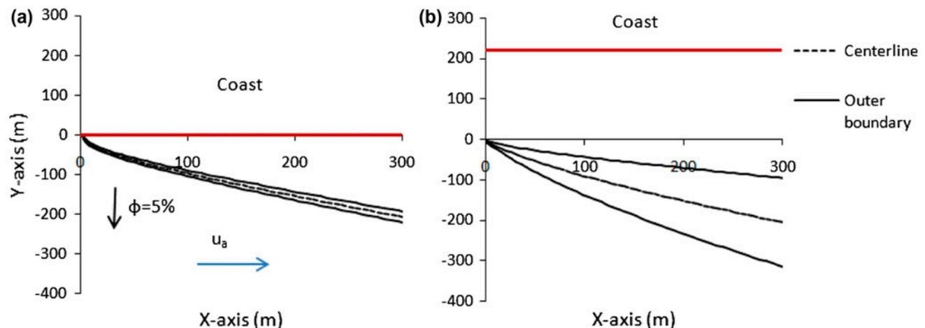
Fig. 7. Plan views of the brine effluent trajectories for scenarios (a) S1 and (b) S2.
