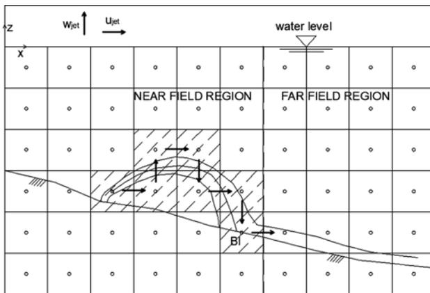
Fig. 8. Schematic representation of the intersected control volumes (dashed lines) of FLOW-3DL with jet axis.
