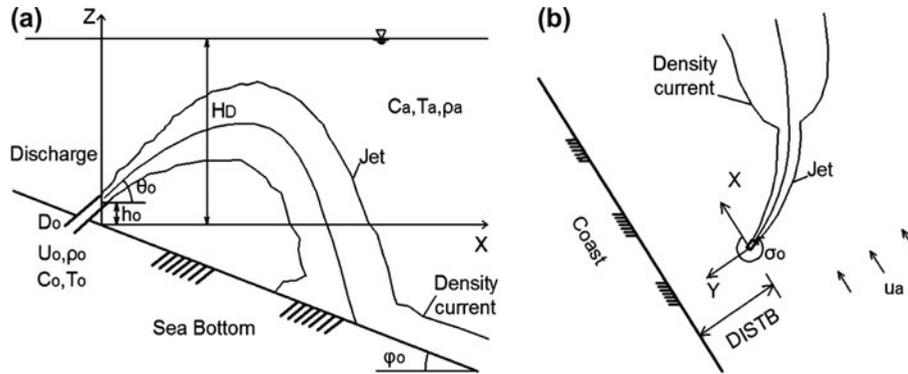
Fig. 1. Schematic representation of a brine discharge into coastal waters; (a) cross section [6], and (b) plan view.
