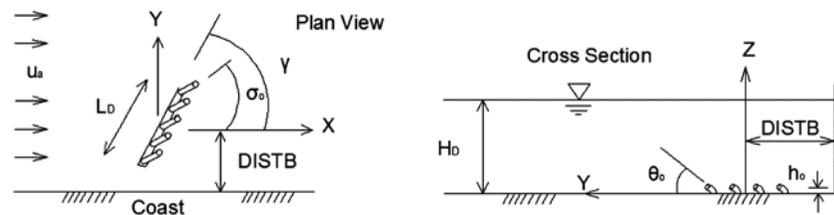
Fig. 6. Plan view and cross-section of an offshore multiport outfall [4].
