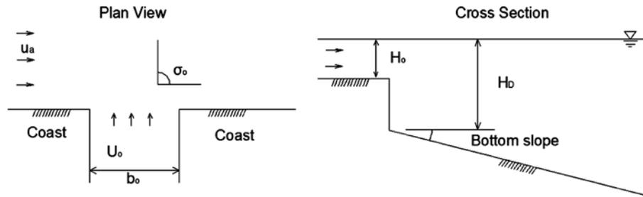
Fig. 4. Plan view and cross-section of rectangular onshore outfalls [4].
