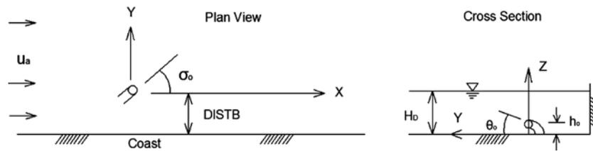
Fig. 5. Plan view and cross-section of an offshore single port outfall [4].
