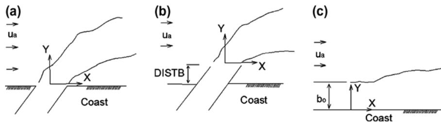
Fig. 3. Types of onshore rectangular outfalls of surface buoyant discharges [4]: (a) flush with bank/shore, (b) protruding from the bank and (c) co-flowing along the bank.
