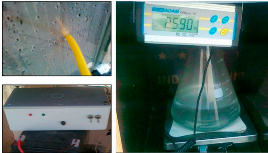
Fig. 3. Thermocouple measuring temperature within the still (top left); storage battery and speed control panel (bottom left); distillate collection flask mounted on digital scale (right).
